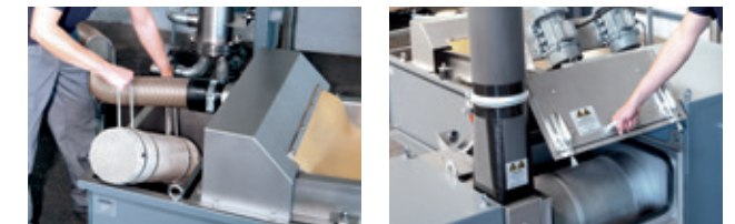
New pellet water removal screen and new pellet centrifuge
