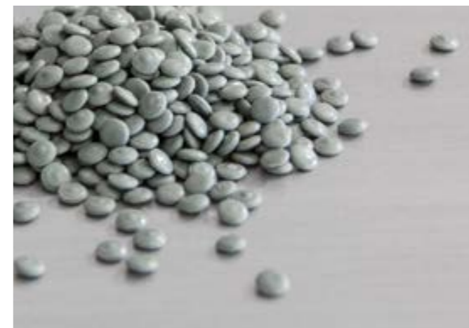
Left: Post-consumer material from the municipal sector has not only heavy contamination but also intense odours. Right: Odour-optimised premium pellets – the result of the combined INTAREMA® TVEplus® technology and subsequent ReFresher process.
