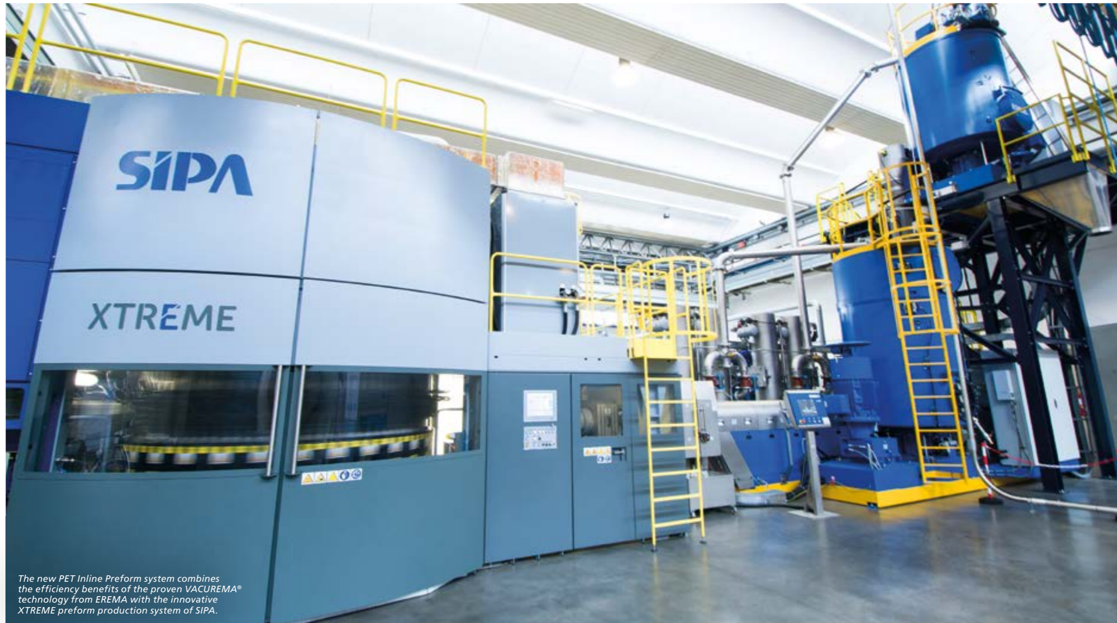
The PET Inline Preform system enables the flexible direct processing of PET flakes to make food contact compliant inline preforms in just one processing step.
