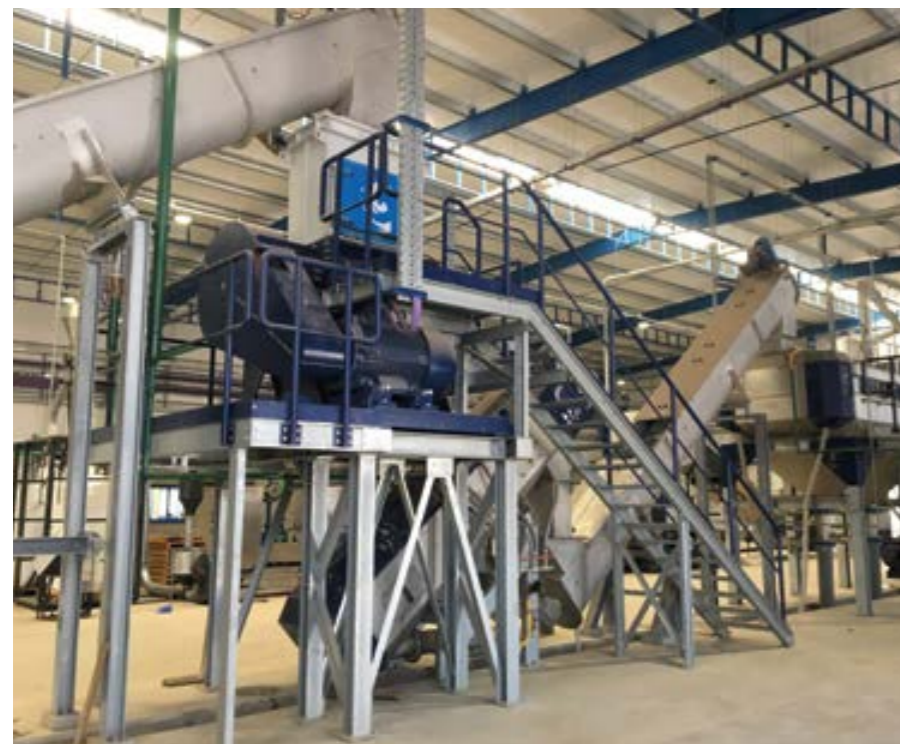
In future, Enviroplast will add post-consumer recycling to its portfolio. For this the company will use a Lindner washing plant with a capacity of 1,000 to 1,500 kg/hour followed by an INTAREMA® 1512 TVEplus® including Laserfilter.
