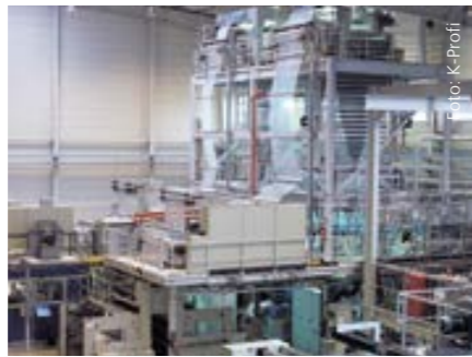
The plastics processor produces 15,000 t/a of flexible films with 3 to 14 layers itself on a total of eight blown film extrusion lines.
